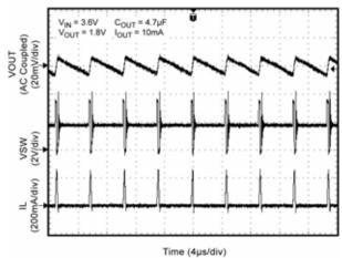
Switching Waveform - Discontinuous Mode
