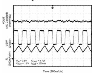
**Switching Waveform - Continuous Mode**
