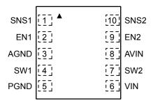
10-Pin 2mm x 2mm Thin MLF $^{\otimes}$  (MT) (Top View)
