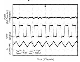
Switching Waveform - Continuous Mode
