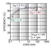
The Figure above shows an efficiency curve. From no load to 100mA, efficiency losses are dominated by quiescent current losses, gate drive and transition losses. By using the Hyper Light Load  $^{\text{TM}}$  mode the MIC23250 is able to maintain high efficiency at low output currents.
