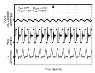
Switching Waveform - Continuous Mode
